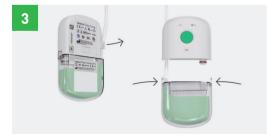
Release tubing at the back of the pump. Press hard on the side-mounted plastic tabs and pull while gently rocking to disconnect the canister. Connect the new canister. You should expect the canister to be a firm fit, this is normal and necessary for maintaining an effective seal.
