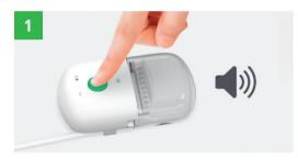
Pause the pump by pressing and holding the green start button, and release after two (2) seconds. The pump will emit two beeps to confirm it is in pause mode.
