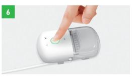
Restart therapy by pressing and holding, and release after two (2) seconds, until the pump activates and the button flashes.
